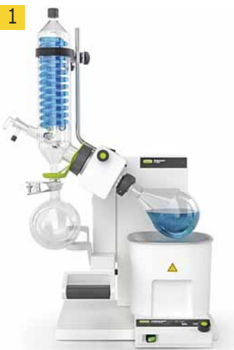
1 Rotavapor® R-300 with heating bath B-301
